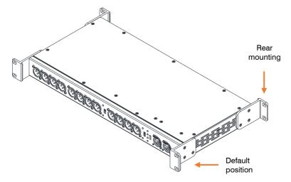
① Only use the M3x8mm countersunk screws provided. Do not use the M3x5mm screws from the standard rack ears.
