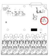
The DIP switches can be found on the right side of the PCB board
