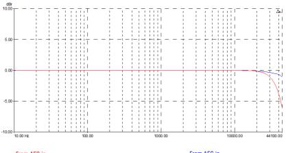
From AES in Switch 1=ON (Sharp Roll-off) From AES in Switch 1=0FF (Slow Roll-off)
