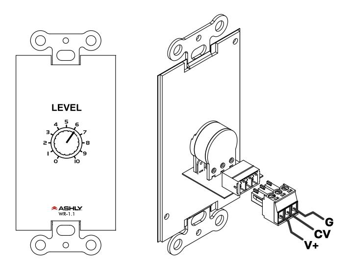
The WR-1.1 is a remote level control for all Ashly products with DC level control inputs on Euroblock connectors. It is designed to fit into a single North American electrical wall box. A decorative cover can be purchased separately at an electrical hardware supplier.
