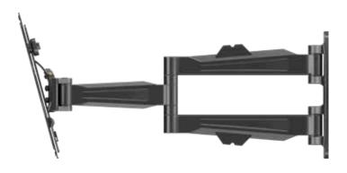
Articulating mount for 13" to 49" displays. Multiple joint arm holds display 2.5" from wall when retracted and 21" when fully extended. Smooth tilt adjustments of +15° (forward) and -5° (back) with a locking knob and 3° side-to-side roll facilitates a variety of viewing angles and perfect positioning. Three attachment points for wood studs and four attachment points for concrete walls provide additional security. Integrated cable management for clean look.
