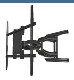
Articulating mount for 37" to 80" displays. Multiple joint arms hold displays 3.4" from wall when retracted and 27" when fully extended. Smooth tilt adjustments of  $\pm 15^\circ$ (forward) and -5° (back) with a locking knob and 3° side-to-side roll facilitates a variety of viewing angles and perfect positioning. Makes a secure installation quick and easy, simply hang the display and turn the pre-assembled securing screws to lock in place. Integrated cable management for clean look.
