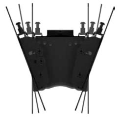
Ceiling mount box and VESA display adapter assembly for 13″ to 46″ dual back to back displays. Attaches to standard 1.5″ threaded extension columns. Continuous tilt of 20° forward with 360° rotation. Makes a secure display installation quick and easy, simply hang the display and turn the pre-assembled securing screw to lock the VESA adapter in place. Compatible with all 1.5″ NPT threaded pipe.
