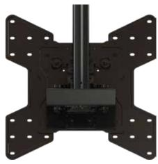
Ceiling mount box and VESA display adapter assembly for 32" to 55"+ displays. Attaches to standard 1.5" threaded extension columns. Continuous tilt of 15° forward with 360° rotation. Makes a secure display installation quick and easy, simply hang the display and turn the pre-assembled securing screw to lock the universal adapter in place. Compatible with all 1.5" NPT threaded pipe.
