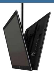
Ceiling mount kit and universal display adapter assembly for dual 37" to 75" displays. Attaches to standard 1.5" threaded extension columns. Continuous tilt of 15° forward with 360° rotation. Makes a secure display installation quick and easy, simply hang the display and turn the pre-assembled securing screw to lock the universal adapter in place. Compatible with all 1.5" NPT threaded pipe.
