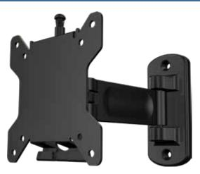
Pivoting mount for 10" to 30" flat panel displays. Swinging arm holds display 2" from wall and extends up to 7.2". Smooth tilt adjustments of 15° forward and 15° back for a variety of viewing angles. Makes a secure installation quick and easy, simply hang the display and turn the pre-assembled securing screw to lock in place. Integrated cable management for clean look.
