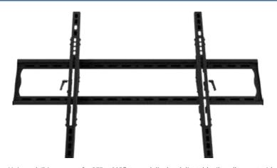
Universal tilting mount for 37" to 90" flat panel display. Adjustable tilt wall mount with Universal hole pattern to fit a wide selection of displays. Smooth tilt adjustments of 15° forward and 5° back with a locking knob for a variety of viewing angles. Makes a  $secure\ installation\ quick\ and\ easy, simply\ hang\ the\ display\ and\ turn\ the\ pre-assembled$ securing screw to lock in place. Open wall plate design provides easy access to wiring
