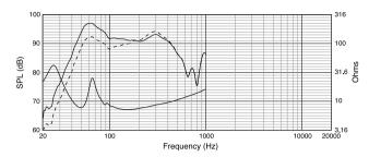
Measured on-axis in half-space ( $4\pi$ , free-space, dotted line), ( $2\pi$  on floor or on wall, solid line), plus Impedance Curve.
