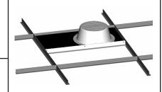
The 1x2 design features an integral T-bar to support the neighboring (cut) ceiling tile.
