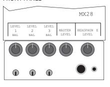
LEVEL 1 - 3: Volume Controls: Adjusts the amount of input signal to the indicated channel. MASTER LEVEL: Master volume control, adjusts the amount of overall signal sent to the Main Right and Left outputs.
