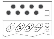
CH 1 - Ch 3 INPUTS: 1/4" unbalanced inputs
