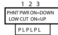
On the left side are the Phantom Power and Low-Cut switches.
