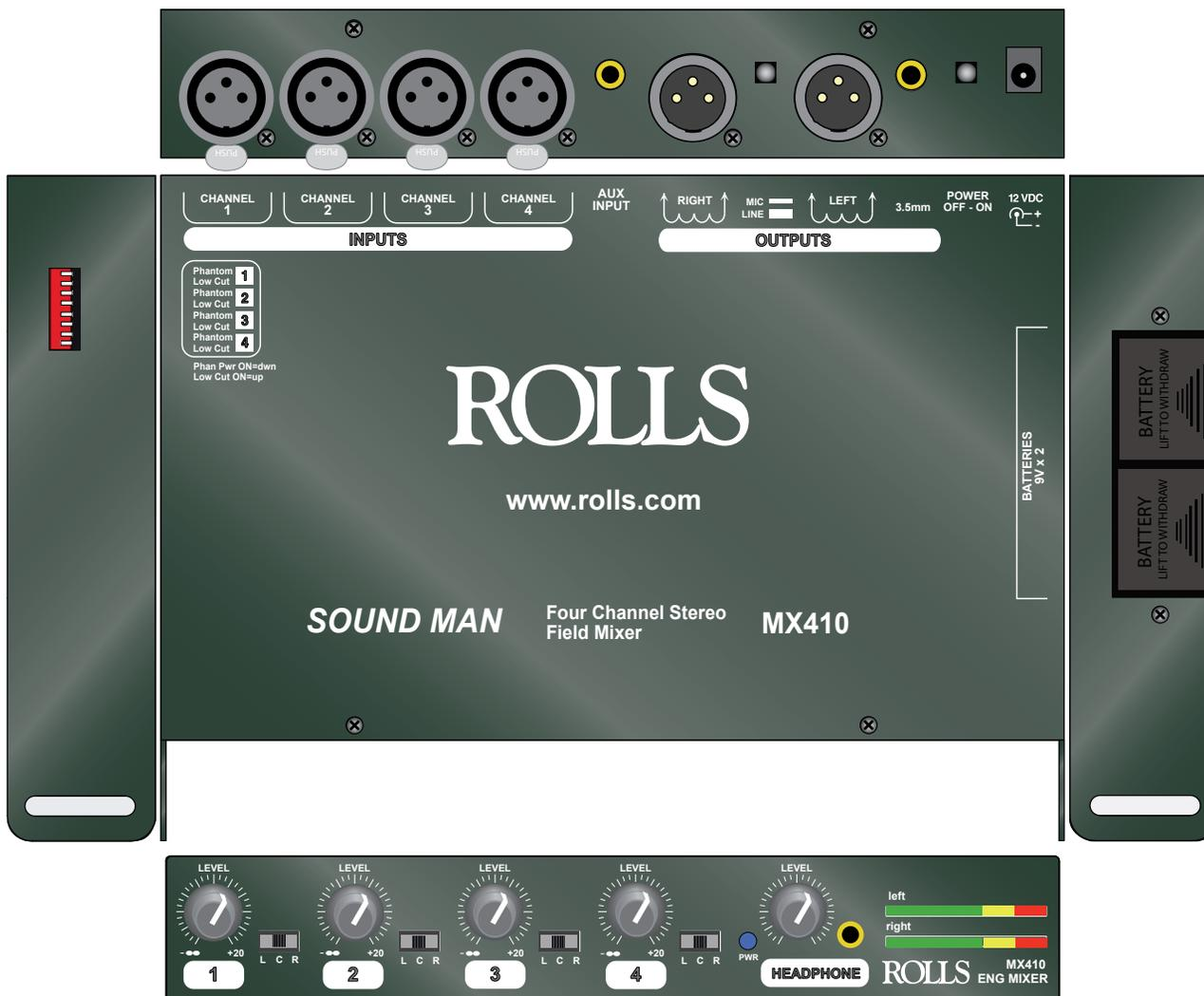
**IMPORTANT NOTICE: DO NOT PLUG MONO (Tip-Sleeve) PLUGS INTO HEADPHONE JACK. DOING SO WILL DAMAGE THE MX410.**
