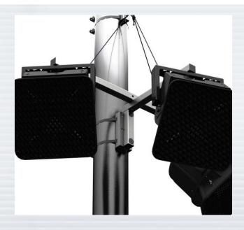
For 6"/154mm diameter and larger poles and columns, use the PM-Mount-6UP. This all-stainless adapter offers a natural finish and supports up to 300 lb./68 Kg, in a vertical load with a 5:1 design factor. It accommodates the PM Series Support Arm, Dual Adapter and includes hardware for their attachment.
