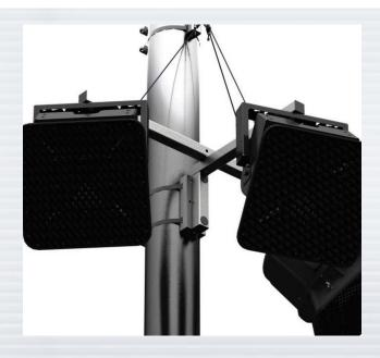
Use the PM-MOUNT-6UP-G for 6"/154mm diameter and larger poles and columns. This galvanized adapter offers a silver / gray finish and supports up to 300 lb./68 Kg, in a vertical load with a 5:1 design factor. It accommodates the PM Series Support Arm, Dual Adapter and includes hardware for their attachment.
