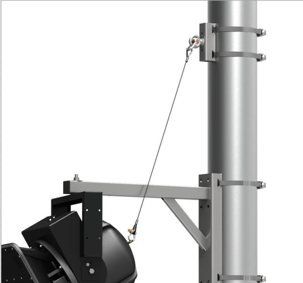
When the pole or column does not offer an adequate way to attach safety cables, specify the PM-Safety-6Down and corresponding band kit. This mount provides a structural method for anchoring safety cables.
