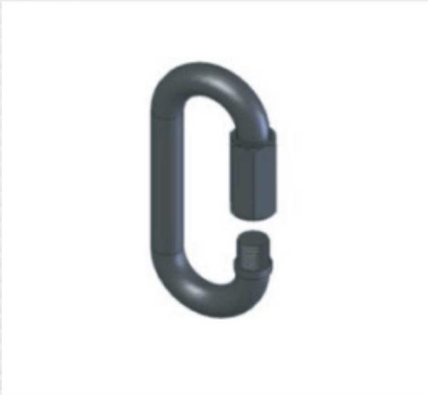
QuickLinks join two closed-end items together, such as wire rope assemblies, turnbuckles and eyebolts quickly and easily. They offer significant working loads for their size and serve as convenient coupling device. Because its side locking turn style has the potential to loosen over time, apply threaded lock when installing for overhead use.
