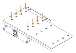
• Align the long mounting ear AA12267 to the threaded holes on the insert bar and joining plate as shown below, and secure it using 6x of the M3x6mm screws provided.
