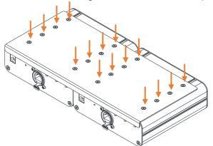
• Align the short mounting ears AA12266 to the threaded holes on the insert bars at each side of the unit, and secure them in place using 8x of the M3x6mm screws provided.
