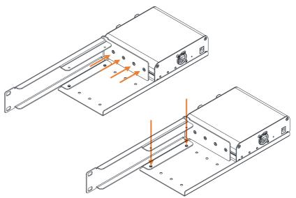
• Align the short mounting ear AA12266 to the threaded holes on the insert bar on the other side of the unit, and secure it using 4x of the M3x6mm screws provided.
