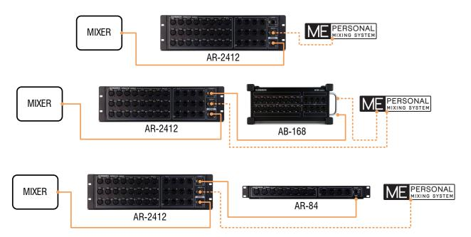
① A maximum of two dSnake remote units can be connected to each mixer's dSnake port.
