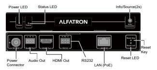
Info/Source (2s) Key: Short press to display/remove on screen information display of decoder; Press and hold for 2 seconds to change the current paired encoder.
