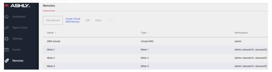
In the software Remotes menu, a remote mixer, DCA, or virtual WR5 can be created, configured, then deployed onto a tablet or mobile device for secure use by a remote operator.
