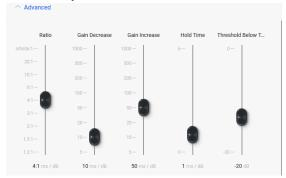
Ratio - This is the ratio of the input level change in dB to output level change in dB. It determines the degree of boost or cut applied to a signal to maintain the target level. The higher the ratio, the closer the signal above threshold will approach the target level. However, a higher level also increases how aggressive the autoleveler maintains that gain.
