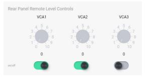
Eight back-panel VCA (voltage controlled amplifier) input pins are used to remotely control the level of assigned inputs or outputs using a simple potentiometer circuit.
