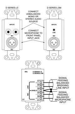
XLR female gold contacts Full size barrier block CASE GROUND, SHIELD (XLR pin 1), + (XLR pin 2), - (XLR pin 3) Phono jacks with gold contacts Full size barrier block +. -. SHIELD 30 Hz to 20 kHz (±1 dB line level) XLR female with gold contacts (1), Phono jacks with gold contacts (2)
