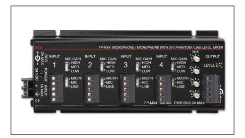
**APPLICATION:** The FP-MX4 is the ideal choice in many applications requiring mixing of microphone and line level sources at preset levels. Power connections are made using either the full-size barrier block terminals or a dc power jack located in one end panel. A second dc power jack is provided on the other end panel for connecting additional FLAT PAK modules.
