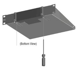
STEP #2 Slide the RACK-UP forward until the screws are seated in the forward position of the cutout. Tighten the screws to secure the unit in the chassis.
