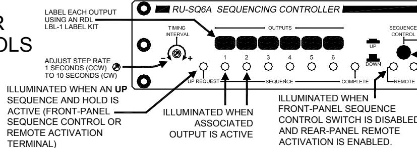
IF ENABLED, LOCKING THE SEQUENCE CONTROL SWITCH IN THE DEPRESSED POSITION CAUSES OUTPUTS TO SEQUENCE UP; RELEASING THE SWITCH CAUSES OUTPUTS TO SEQUENCE DOWN.
