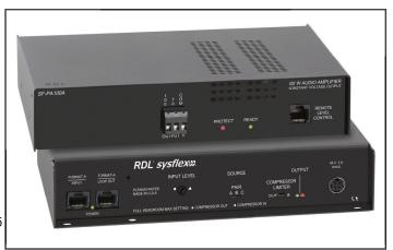
**APPLICATION:** The SF-PA100A is an audio power amplifier that receives three audio channels on an RJ45 Format-A connector. A selector feeds Pair A, Pair B or Pair C audio to the amplifier that provides a 70 V or 100 V constant voltage amplified output. At the normal gain setting, the output provides 100 watts for an audio level of +22 dBu. The three Format-A pairs feed through to the LOOP OUT jack to feed additional amplifiers or other Format-A receivers.
