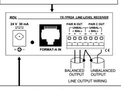
Connect external power if unit is not receiving power from the connected sender. Maximum load current is 200 mA for the RJ45 jack. Power supply must be rated for more than total connected load. The **PWR** LED indicates the presence of valid power.
