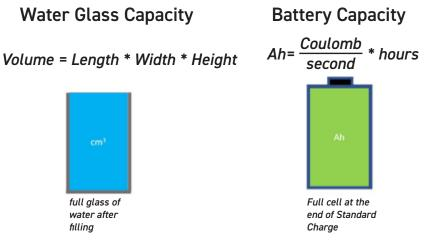
Figure 1.1: Comparing Battery Charge to a Glass of Water
