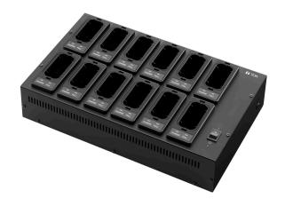
The TOA BC-5000-6 and BC-5000-12 are dedicated battery chargers for the WM-5225 and WM-5265 Wireless Microphones, WM-5325 Wireless Transmitter, and the WT-5100 Portable Receiver. Both chargers work with the optional AD-5000-6 AC Adapter. The BC-5000-6 and BC-5000-12 employ a quick charging system for nickel-metal hydride (Ni-MH) batteries, allowing up to 6 or 12 units to be fully charged within 3 hours.
