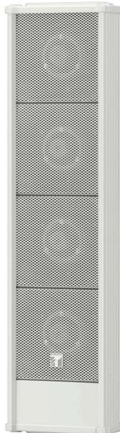
The HA-1030EN is composed of multiple horn speakers positioned in an array. It is a highly efficient speaker. Clear voice can be transmitted to a distant place without acoustic correction. The built-in high-pass filter cuts the bass that can damage the speaker. A double drip-proof structure, and a salt-resistant paint finish, it has excellent durability in an outdoor permanent environment.
