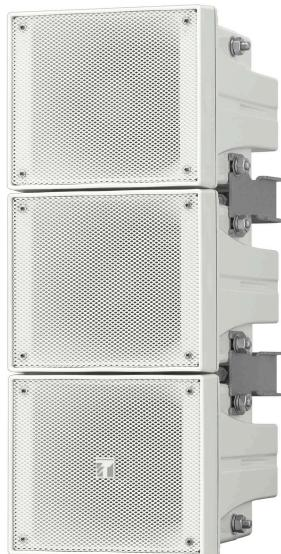
The HA-2120EN is composed of multiple horn speakers positioned in an array. It is a highly efficient speaker. Clear voice can be transmitted to a distant place without acoustic correction. The built-in high-pass filter cuts the bass that can damage the speaker. Drip-proof structure, and a salt-resistant paint finish, it has excellent durability in an outdoor permanent environment.
