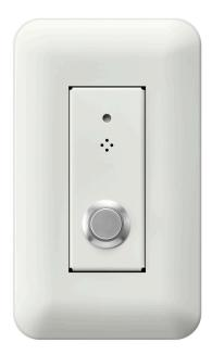
The IP-A1MP is a microphone panel that is equipped with a microphone, an activation switch and a status indicator. It can be installed with a standard electrical box as surface or flush mounting. This panel can be used as a two-way conversation or an audio monitoring microphone when used in conjunction with IP-A1 series devices.
