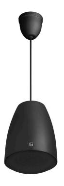
The Q-PE-304BK is a pendant speaker designed for ceiling suspension installations. Considered in architectural design, it can blend in with lighting equipment. A directly-attached 5 m (16.4 ft) cable allows the speaker to be suspended from the high ceiling. The Q-PE-304BK is driven on both high-impedance (100 V and 70 V) and low-impedance (8 Ohm) lines. The impedance can be easily changed at the upper side of the speaker. The speaker is easy to repaint so as to meet a wide range of design needs.
