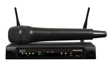
The TOA's TRANTEC S4.10 series Wireless Microphone system is designed for use on the UHF frequency band, and suitable for vocal or speech reinforcement applications. It features a compander circuit which minimizes the influence of ambient noise.S4.10-HD includes a wireless handheld microphone and a diversity receiver.
