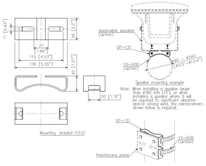
Example of mounting reinforcement
