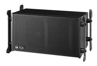
The SR-C8L is a 2-way line array speaker featuring wave front control technology which creates a sound field with high sound clarity and uniform sound pressure. Recommended digital speaker processor is the DP-SP3. It can be converted into the bi-amplifier drive system by changing the internal connection.
