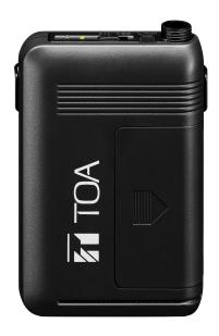
The WM-5325 wireless transmitter has been manufactured for use with a UHF system. It is for use in speech reinforcement applications. Thanks to the PLL-synthesizer system, 64 different operating frequencies are made available. A high output power ensures stable radio signal transmission.
