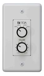
Remote Control Panel is a remote control switch/volume panel designed to be used with the MA-725F or MM-700F amplifiers. Provides remote select input source and adjusts volume levels through an Ethernet cable. It can be mounted in a 1-gang electrical box.
